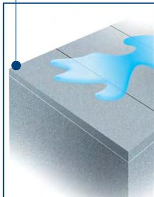
CDS Single piece lids have a unique tongue and groove rim reducing lateral movement and leaks
